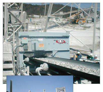
Introducing JBLCo's newly designed product sampler, the QC-360. This quality control sampler developed, primarily, for the Aggregate Industry, will allow for the collection of reliable results for quality control purposes.
