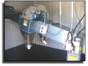
A CLEAN SWEEP® secondary sampler is positioned on the CMF conveyor to take subsamples. Its highly flexible design can be configured to sweep samples to discharge points on either or both sides of the CMF conveyor. Individual save sample containers can be positioned at these points or a multiple container sample carousel may be installed.
