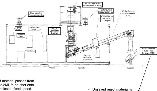
Crushed material passes from the SampleMill™ crusher onto a fully enclosed, fixed speed **Crushed Material Feeder**
